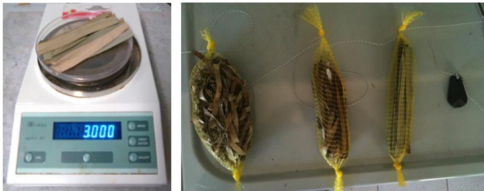
Figure 20 - Analytical balance (left) and leaf packs of P. australis leaves ready for field introduction (right).
