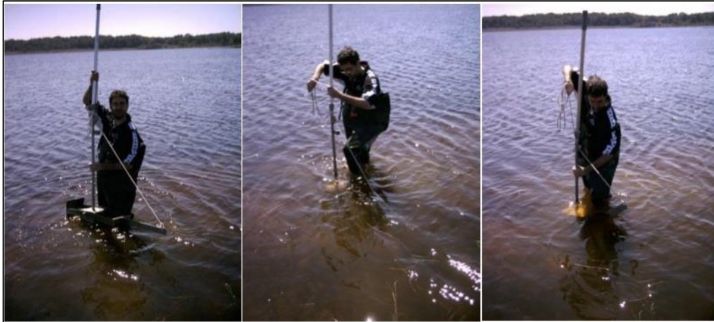
Figure 15 - Phases of sediment sampling by means of the box corer (Sangiorgio et al., 2009).
